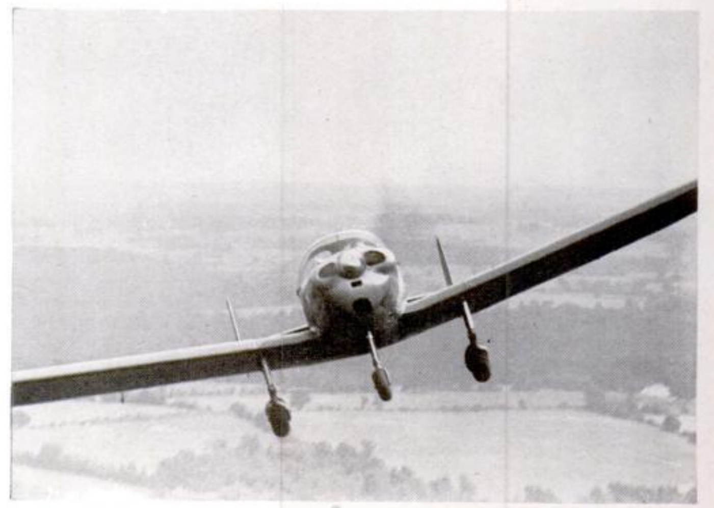
Banking the Ercoupe can never be done so severely as to put plane into a spin. Notice the double rudder, which gives greater stability, and tricycle landing gear.
